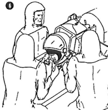
THREE MEN ARE REQUIRED TO REMOVE PILOT ONE ON EACH SIDE AND ONE ASTRIDE THE COCKPIT IN FRONT OF PILOT
