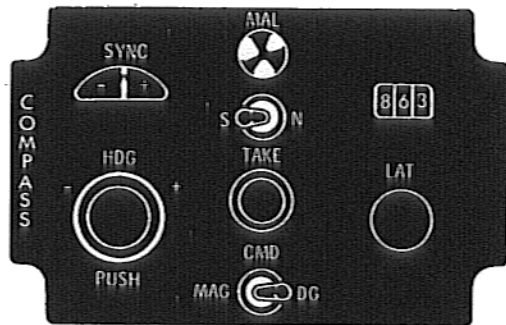
DETAIL B FLIGHT REFERENCE SYSTEM CONTROL PANEL
