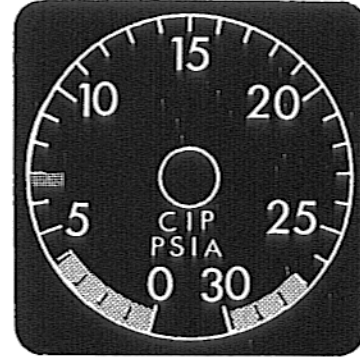
COMPRESSOR INLET STATIC PRESSURE GAGE
