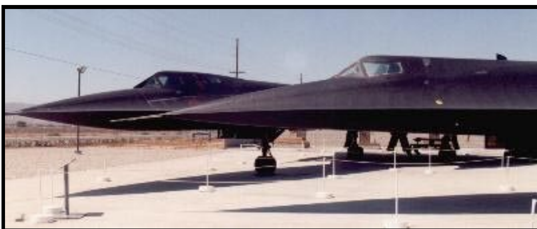
A-12 and SR-71(background), nose to nose. Note extra window behind canopy on SR-71
