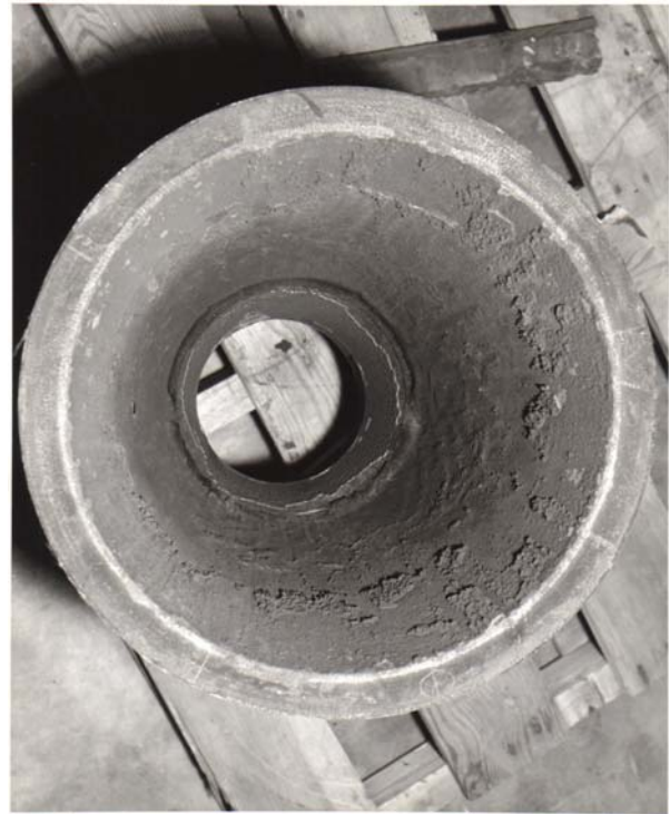
Figure 23. Post-test view of nozzle exit cone.
