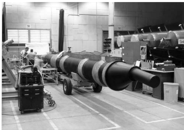
Figure 9. Completed application of aerodynamic rings.
