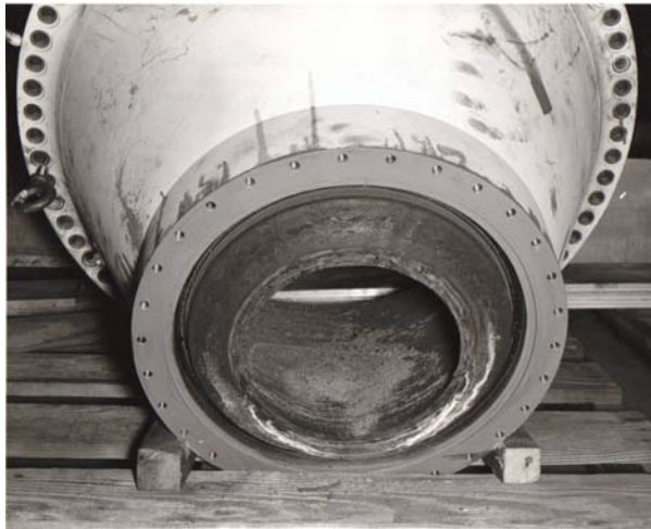
Figure 20. External post-test view of aft closure.
