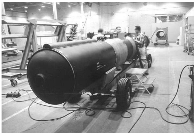
Figure 7. A second aerodynamic ring is applied.
