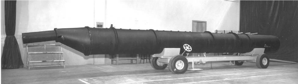
Figure 5. D-21B Avanti booster assembly on the manufacturing floor.
